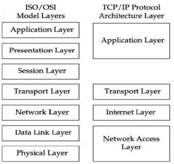
Figure 5.6 A comparison of TCP/IP and ISO/OSI models.
